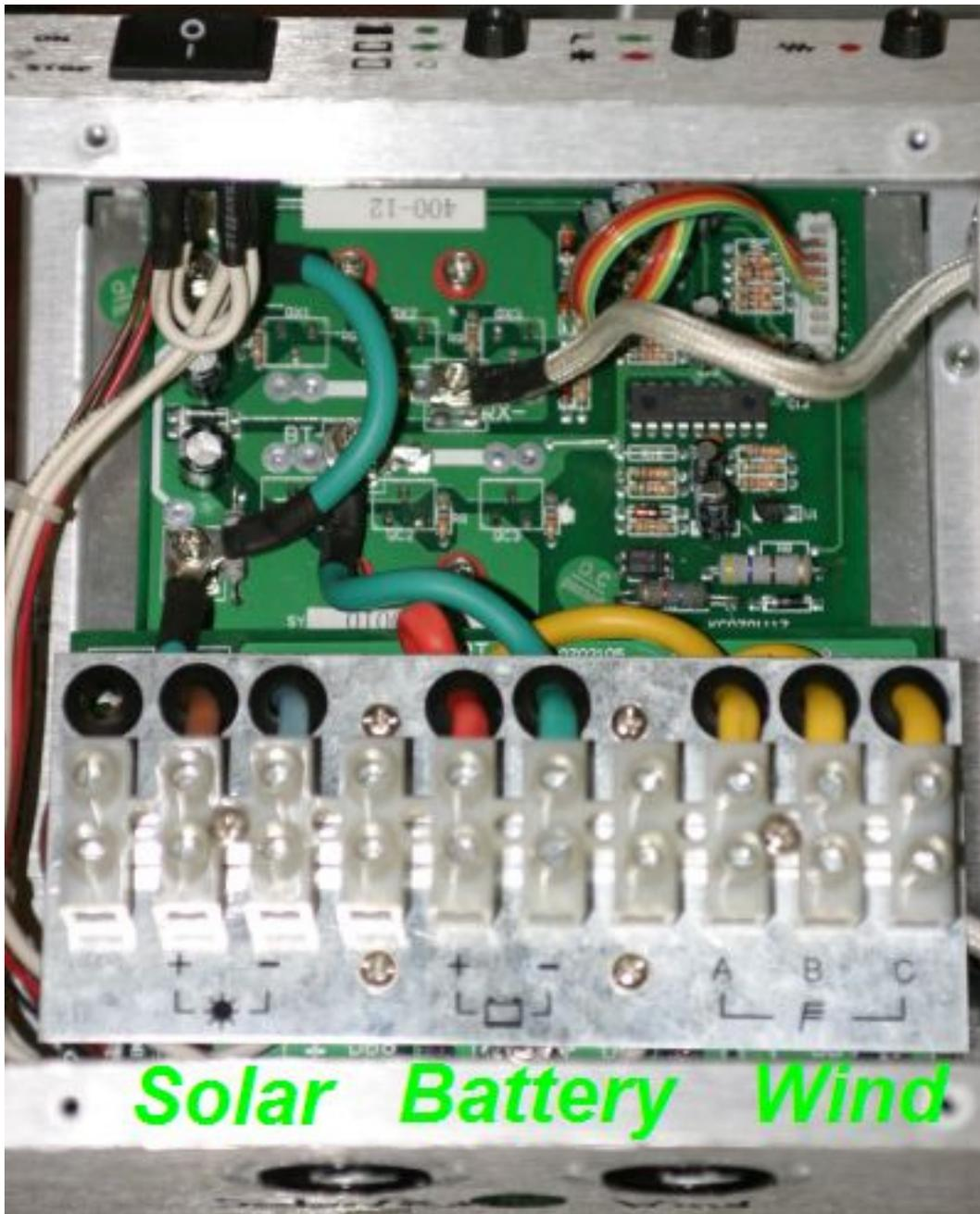
3. Install a minimum 100amp breaker switch for the 3-phase AC wires from generator, and connect the wind generator 3-phase AC wires from breaker switch to controller's "WIND" terminals (no sequence).
