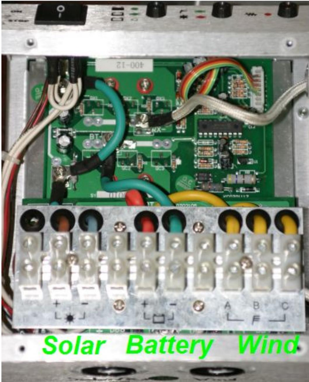
3. Connect the wind generator 3 phase AC output to “WIND” terminal.
