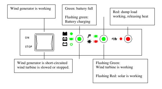
Note: Output voltage of some solar panels is much higher than 12V or 24V, and this may trigger the dump load early or make battery light show "solid green". Please make sure the maximum output voltage of solar panels is below 14V for 12V controllers and below 28V for 24V controllers.
